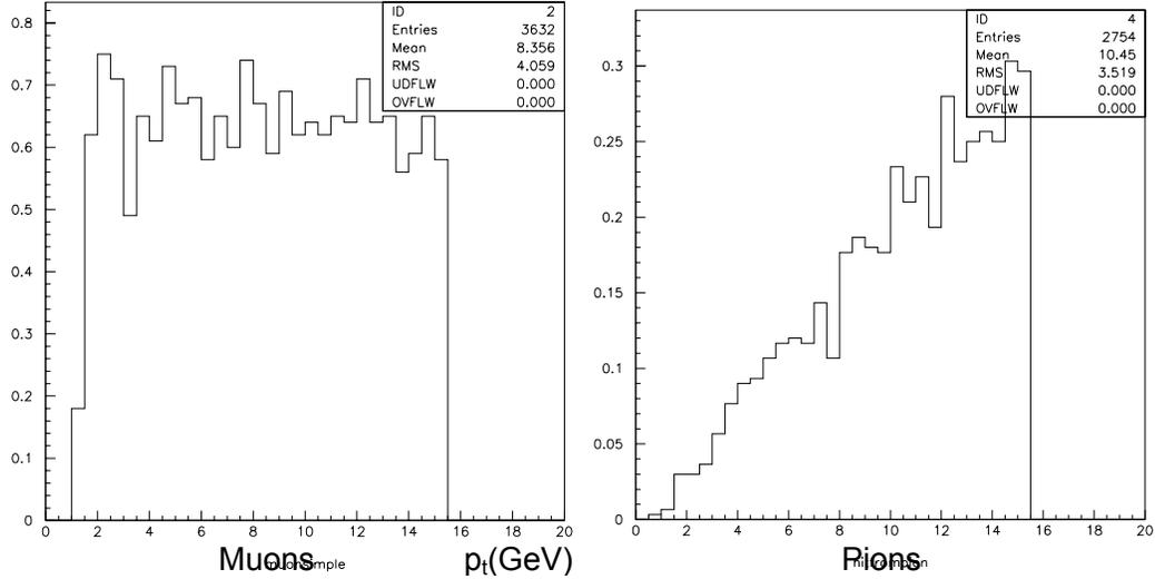
**Fig.4 Fractions of muon and pion with hits in the MTD vs pT without additional cuts. MTD has 73% of the coverage avoiding the gaps of the magnet return iron bars**
