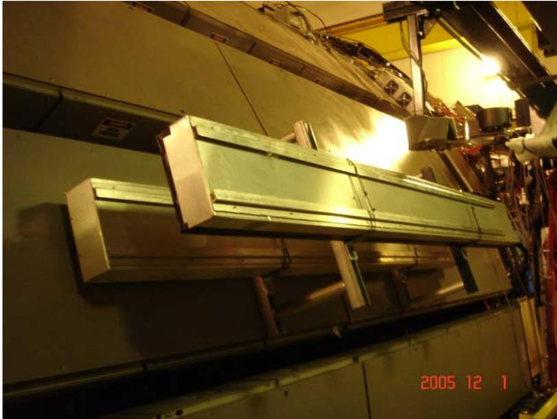
**Fig.10 a test MTD using two spare CTB trays. The trays are attached to the HV box outside the iron bars and are separated by 35cm radially.**
