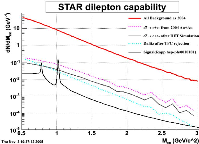
**Fig.2 Dielectron Invariant Mass from simulation based on run4 data. This shows that  $c+\bar{c} \rightarrow e+e-$  dominates after background rejection from gamma conversion and Dalitz decays**
