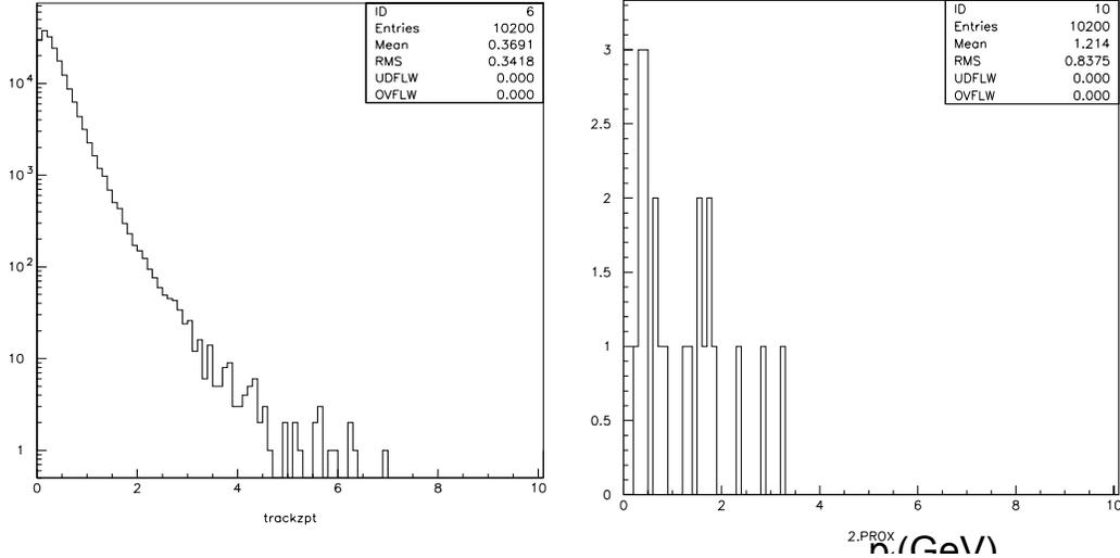
**Fig.9 HIJING input particle pT distribution and the pT distribution of particles matching with MTD hits, which includes random coincidence.**
