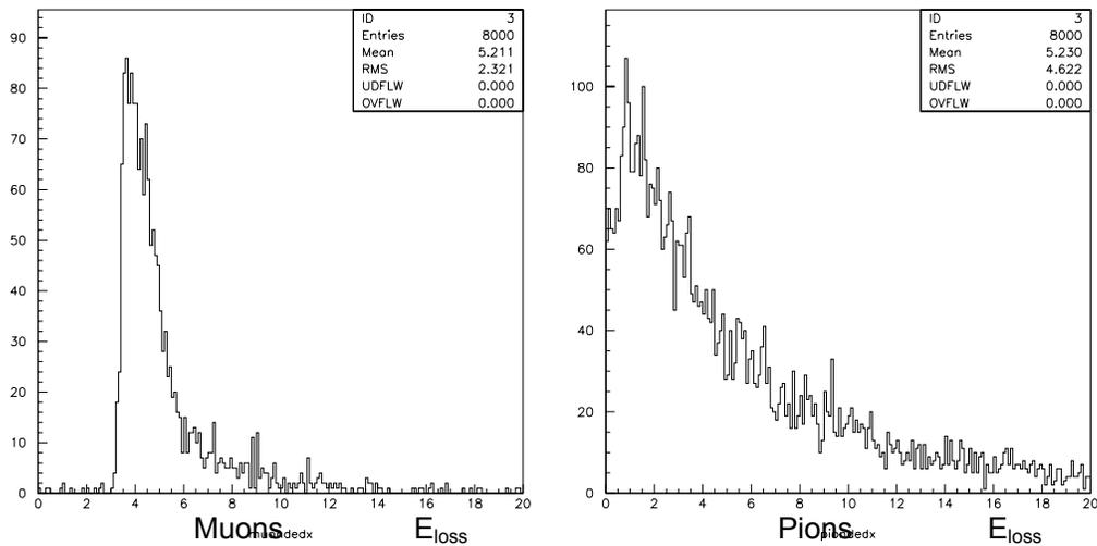
**Fig.7 The muon  $dE/dx$  in MTD and the  $dE/dx$  of all particles associated with a primary pion.**
