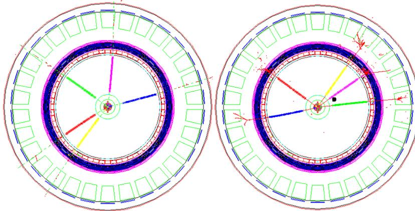
**Fig.3 Examples of single muon and pion tracks in TPC**
