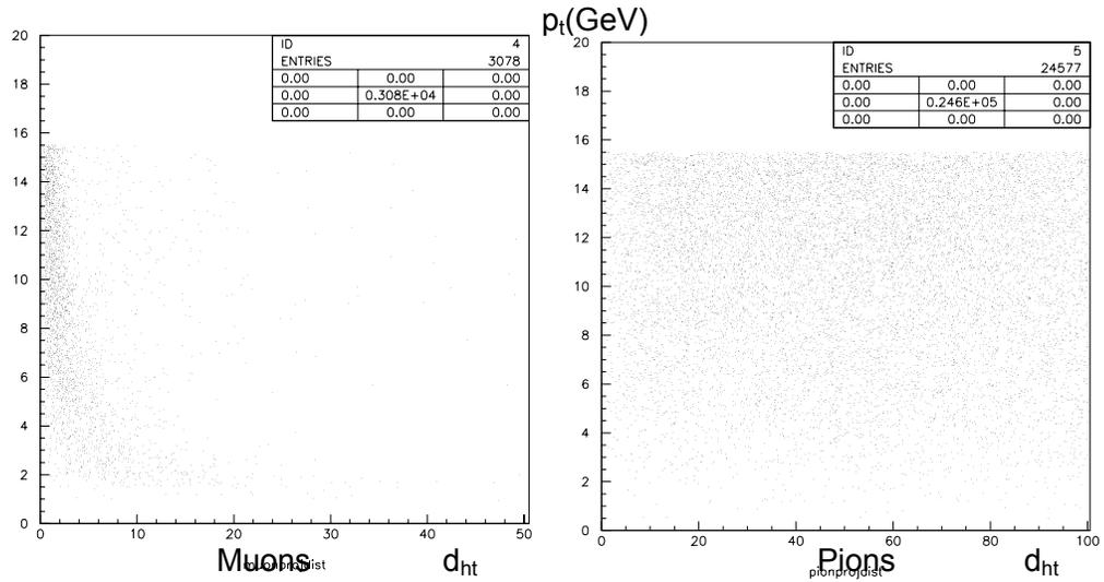
**Fig.6 Distance between the hit position in MTD and a simple helix projection of the track from TPC.**
