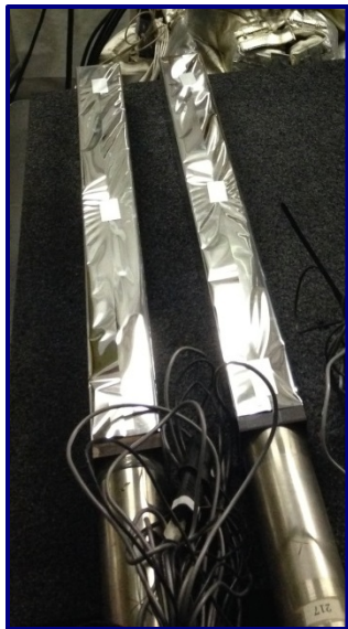
Replacement of PMT and bases
