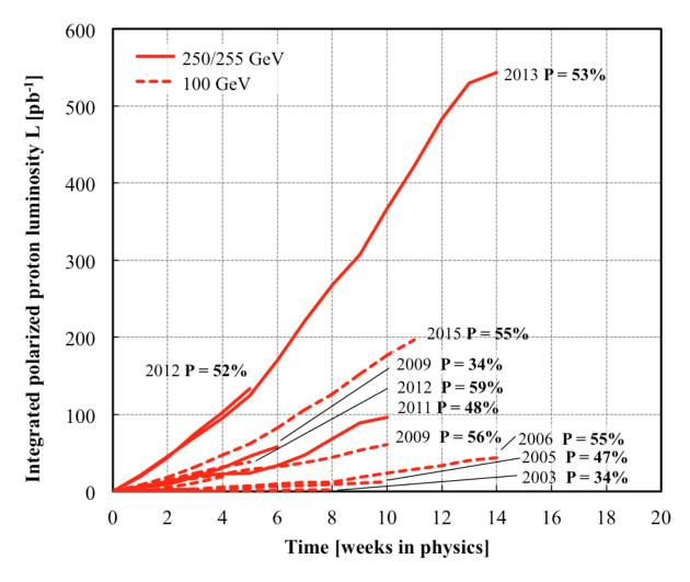
Consistent improvement in delivered luminosity and beam polarizations
