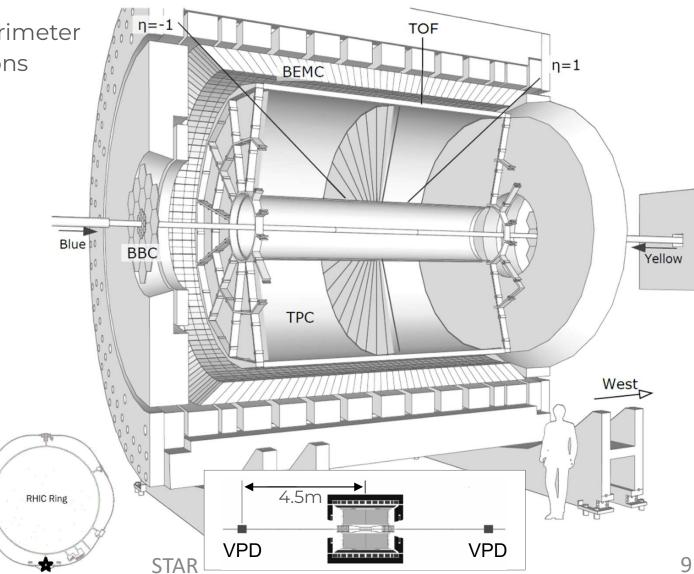
Barrel Electromagnetic Calorimeter 60m² |η|<1.0
