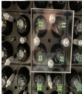
Step B: Gluing SiPM carrying boards to LG (4 SiPM/tower, 5984 total)
