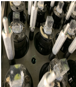
Step A: Gluing four light guides/mixers at the end of WLS bundles
