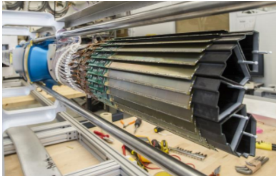
Figure 2.8: Picture of one half of the Pixel detector showing its five trapezoidal sectors. Each sector supports four ladders, three outside (visible) and an inner one. Also shown is the Pixel support and insertion mechanism.
