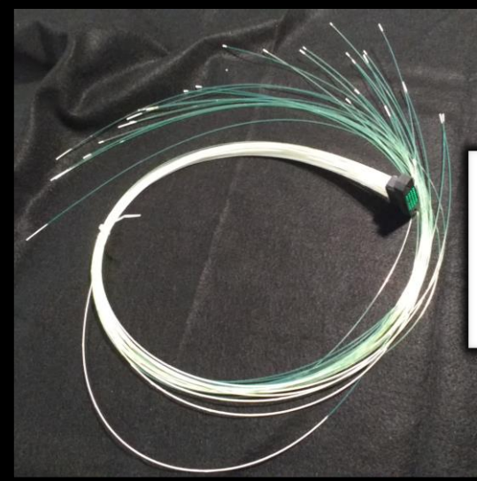
Fiber bundle containing 31 wavelength-shifting fibers
