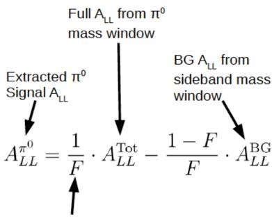
$F=\pi^0 \mbox{ Purity: fraction of events in } \pi^0 \mbox{ mass window which are likely } \pi^0 s$
