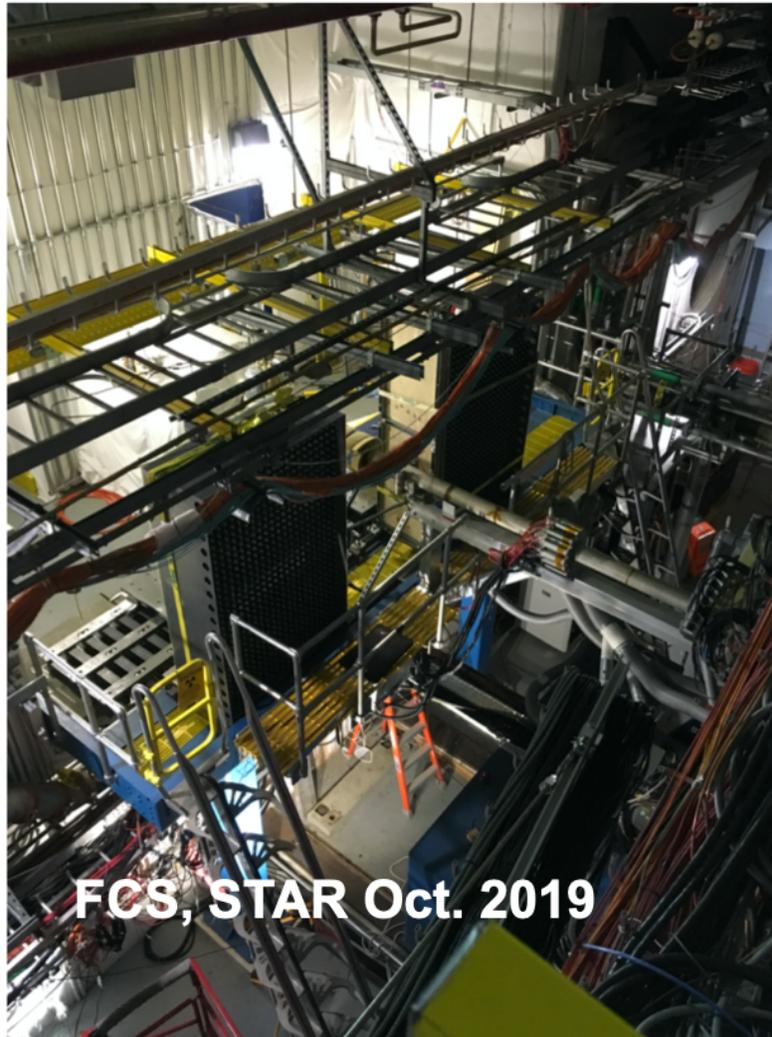
**Figure 91:** A view of the installed forward ECal detector halves, left and right from the beam pipe.
