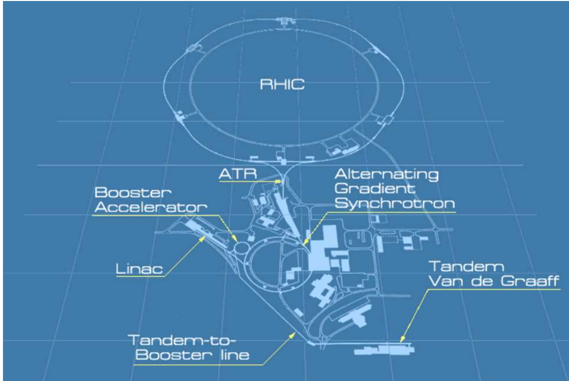
Figure 3.1: The RHIC complex. Protons follow a path through the Linac, Booster, AGS, ATR (AGS to RHIC line) and into the RHIC ring. The Tandem Van de Graaff generator is used in the acceleration of heavy ions.
