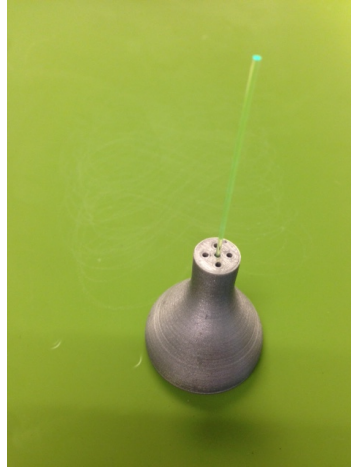
Figure 34: Fiber holder and fiber on top of the green polishing sheet of the second lowest grit size.
