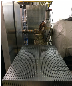
Fig : Stacking layers of absorbers with scintillators sandwiched (left), Installing WLS bars (middle), Installing LED (right)
