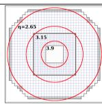
FMS is a lead-glass electromagnetic calorimeter
