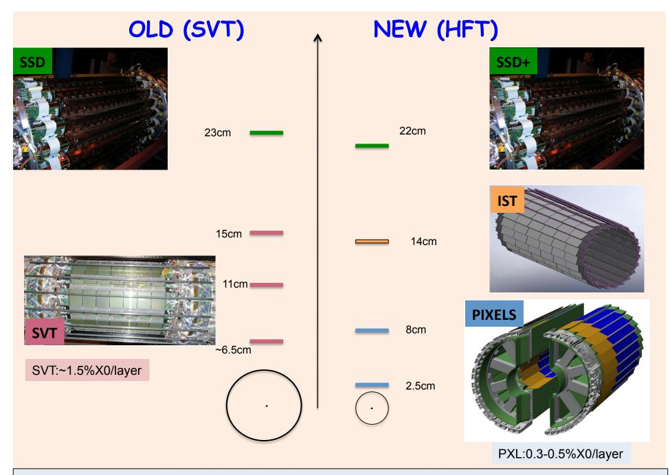
Detector resolutions differ by a factor of two but pointing by a factor of ten.
