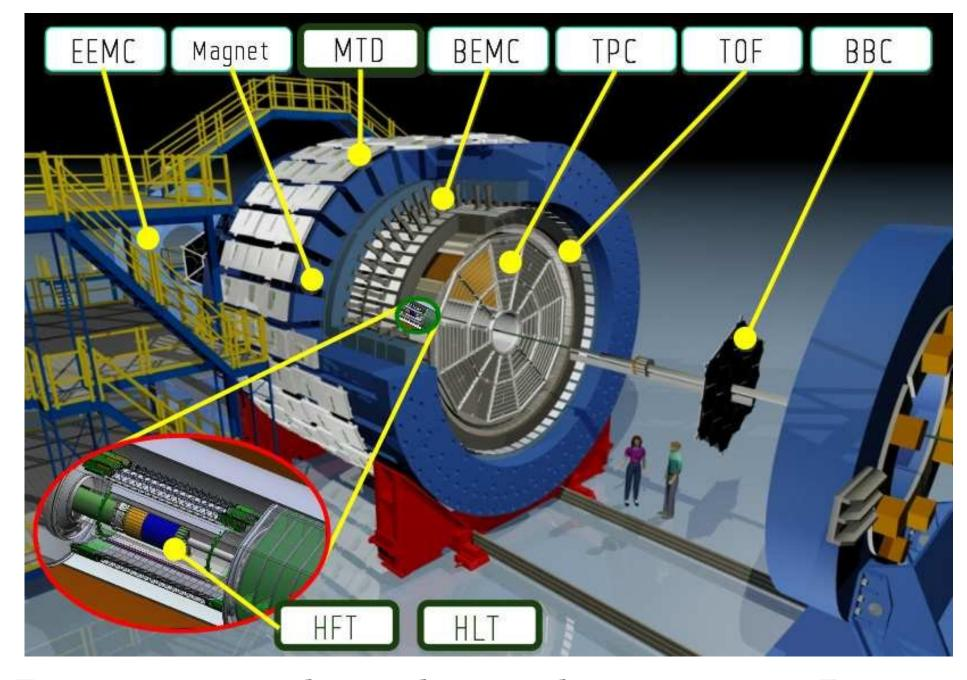
Detectors used in the analysis: Time Projection Chamber (TPC), Time-of-Flight (ToF) and Heavy Flavor Tracker (HFT)
