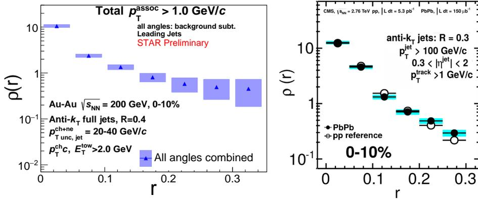
**Figure 1:** The total differential jet shape (greater than 1.0 GeV/c) for leading anti- $k_T$  full jets with  $20 < p_T^{\text{jet}} < 40$  GeV/c of size  $R = 0.4$  in the 0-10% most central Au+Au events at 200 GeV (left) and a similar measurement by the CMS Collaboration at  $\sqrt{s_{\text{NN}}} = 2.76$  TeV (right).
