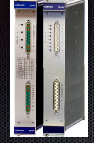
controlling 40 channels of low voltage power for the hadron (HCAL) and electron (ECAL) calorimeters
