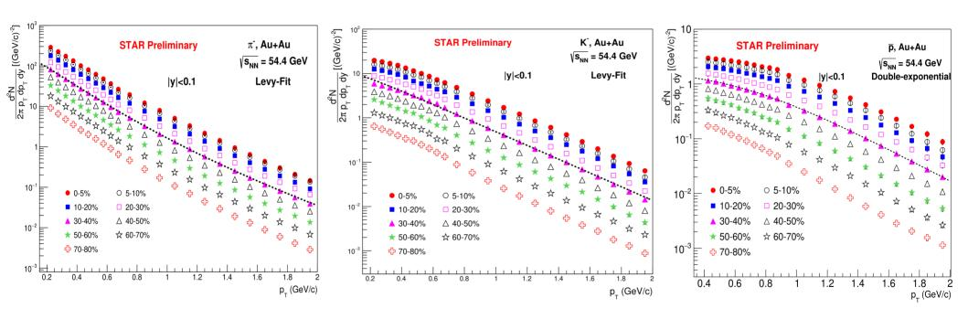
The yields from TPC are obtained for  $p_T < 0.75$  GeV/c for  $\pi^-$  and  $K^-$ , and  $p_T < 0.85$  GeV/c for  $\overline{p}$ . The yields from TOF are obtained within rapidity |y| < 0.1 for  $p_T > 0.7$  GeV/c for  $\pi^-$  and  $K^-$ , and  $p_T > 0.9$  GeV/c for  $\overline{p}$ .
