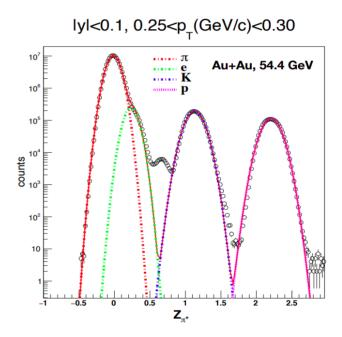
Particle identification is accompalished in the TPC by measuring the <dE/dx>. The dE/dx distribution, for a given particle type, can be transformed to the z variable which is given by  $z_X = \ln\left(\frac{\langle dE/dx \rangle}{\langle dE/dx \rangle_X^B}\right)$ , where X is particle type and B is Bichsel function.
