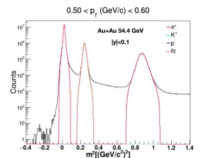
The raw yields from TOF are obtained using the variable mass square (m<sup>2</sup>), given by,  $m^2 = p^2 \left( \frac{c^2 T^2}{L^2} - 1 \right)$
