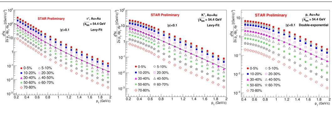
The yields from TPC are obtained for  $p_T < 0.75$  GeV/c for  $\pi^+$  and  $K^+$ , and  $p_T < 0.85$  GeV/c for p. The yields from TOF are obtained within rapidity |y| < 0.1 for  $p_T > 0.7$  GeV/c for  $\pi^+$  and  $K^+$ , and  $p_T > 0.9$  GeV/c for p.
