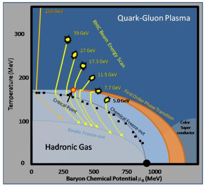
The main idea behind the BES program is to vary the collision energy and look for the signatures of the QCD phase boundary and QCD critical point.
