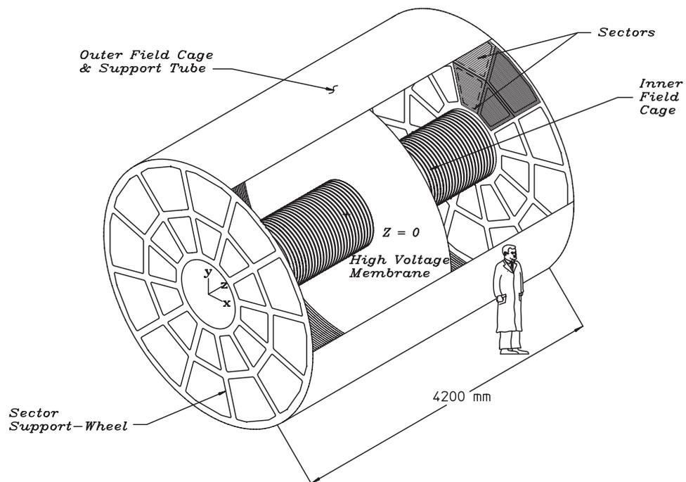
Figure 2.3: Diagram of the STAR TPC showing the main components as well as the scale. From [33]
