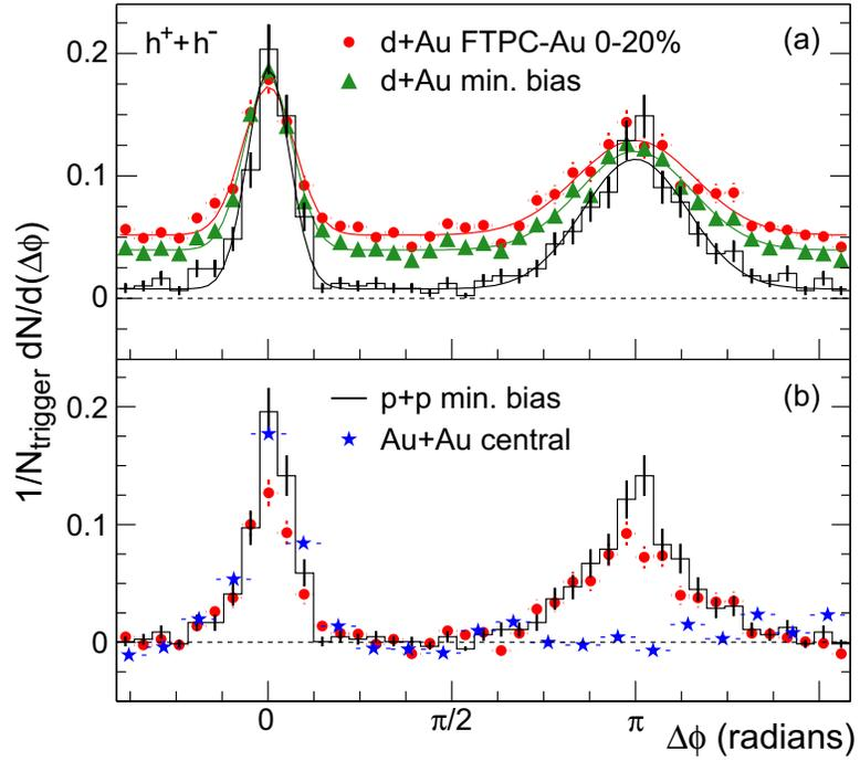
Figure 1.8: Azimuthal dihadron correlations in STAR. Strong quenching of the away side jet is seen in Au+Au collisions but not p+p or d+Au. Lack of suppression in d+Au rules out cold nuclear matter effects on jet suppression [12].
