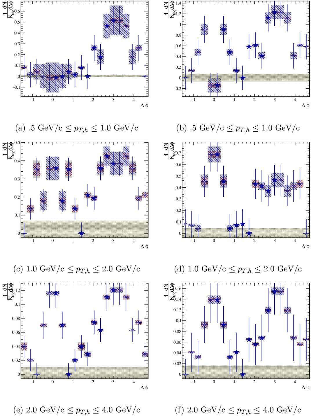
Figure 4.9: Background subtracted NPE-h correlations for 40-60% centrality events. Trigger  $p_T$  is  $4.0 \text{ GeV}/c \leq p_{T, \text{trig}} \leq 6.0 \text{ GeV}/c$  for the left column and  $6.0 \text{ GeV}/c \leq p_{T, \text{trig}} \leq 9.0 \text{ GeV}/c$  for the right column.
