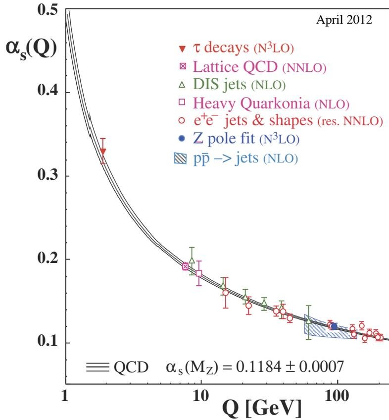
Figure 1.1: Several measurements of the strong coupling constant  $\alpha_s$  showing how it varies with energy scale. Decreasing coupling strength as the interaction energy goes up is consistent with predictions of asymptotic freedom [3].
