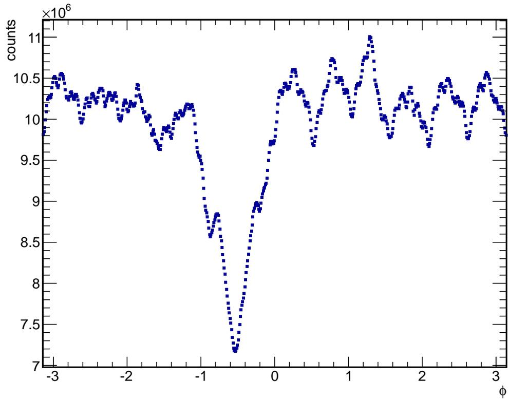
Figure 4.1: The azimuthal angular distribution of all tracks in Run11 Au+Au collisions at 200 GeV. Periodic bumps can be seen from the sector boundaries, as well as a dip in the poorly performing sector.
