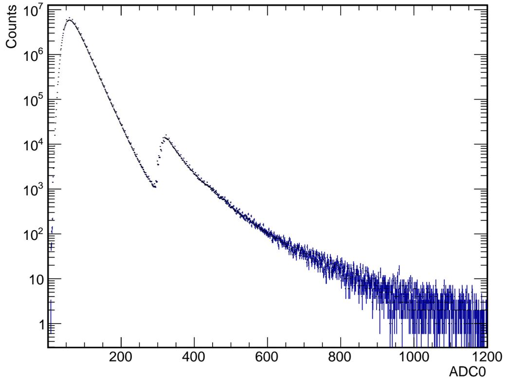
Figure 3.5: ADC0 for primary tracks in NPE18 triggered events. Turn on of the NPE18 trigger is apparent around 325 ADC counts.
