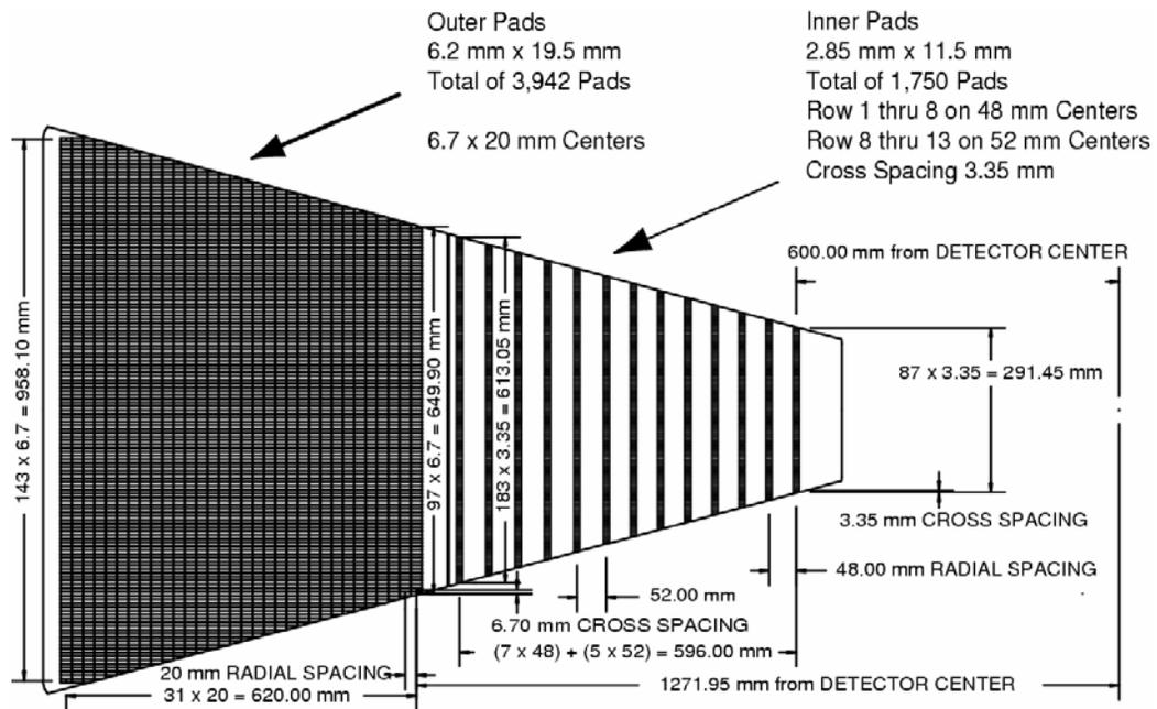
Figure 2.5: Schematic of one TPC pad plane. The difference in spacing between inner and outer pads can be seen [33].
