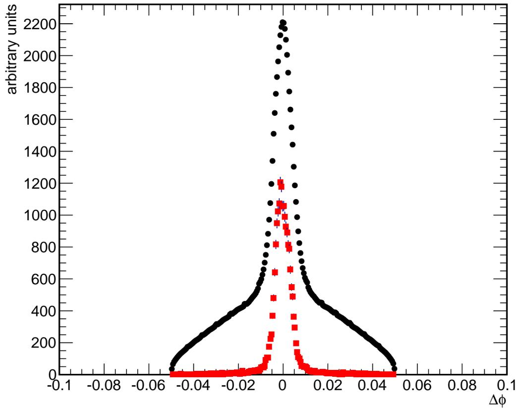
Figure 3.6:  $\Delta\phi$  between the TPC and BEMC for all matched primary tracks (black) and identified electrons (red). Y-axis is arbitrary units scaled to show all tracks and electrons on the same figure. Matching is better for electrons and we cut on such that  $|\Delta\phi| \leq .013$ .
