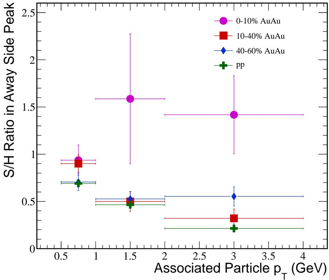
Figure 4.16: Ratio of yields in shoulder region to head region in NPE-h correlations for trigger electrons have  $4.0 \text{ GeV}/c \leq p_T \leq 6.0 \text{ GeV}/c$ . A larger ratio indicates a wider peak.
