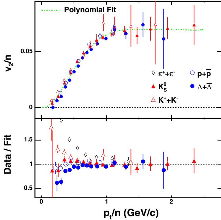
Figure 1.6: Identified particle  $v_2$  as measured in 200 GeV Au+Au minimum bias collisions in STAR scaled by the number of constituent quarks. Common trend across hadrons is evidence for hadronization from coalescence of thermalized quarks [9].
