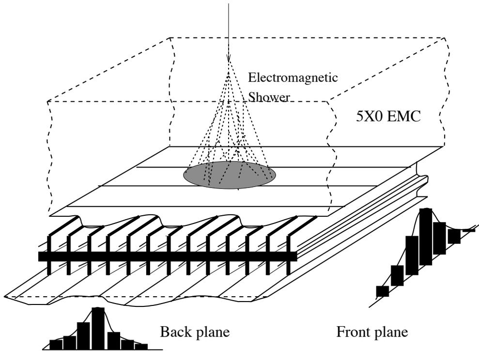
Figure 2.7: Illustration of the function of the BSMD detector. Particle enters the tower (at top) and develops into a shower which registers hits in the  $\eta$  and  $\phi$  directions in the BSMD [32].
