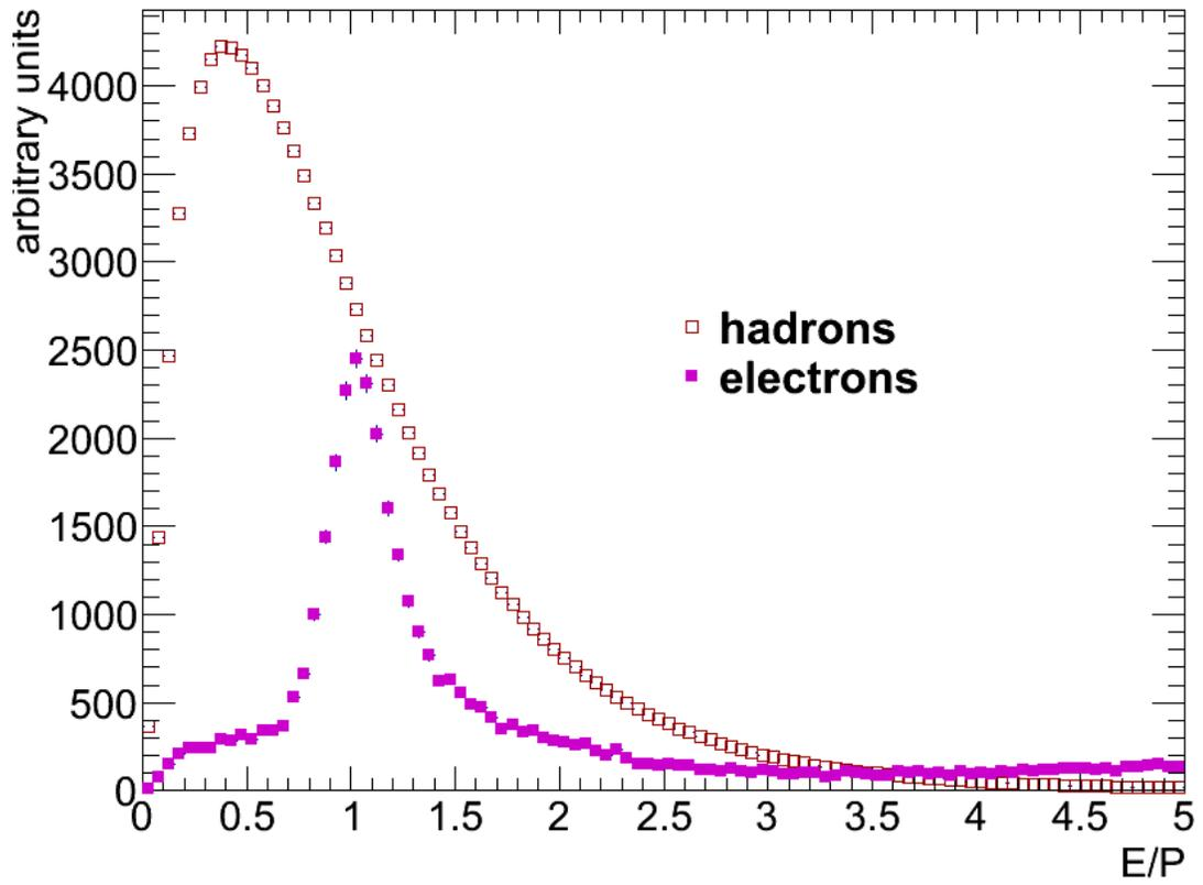
Figure 3.9:  $E/p$  for points in the BEMC for electrons (without  $E/p$  cut applied) and hadrons. Scale is arbitrary to show both cases. Electron cut is set  $.5 \leq E/p \leq 1.7$ .
