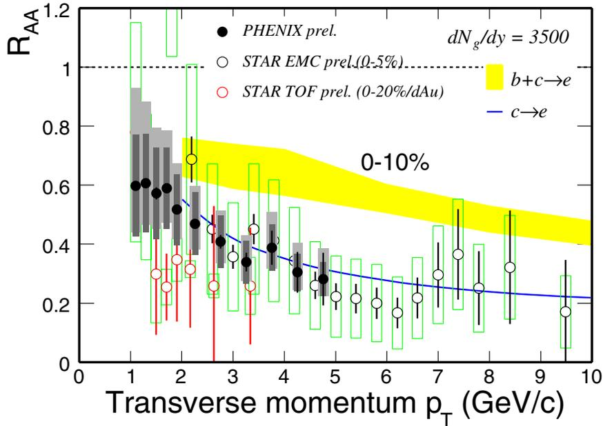
Figure 1.9: Non-photonic electron  $R_{AA}$  from central Au+Au collisions measured by STAR and PHENIX. The theoretical curves show expected suppression due to radiative energy loss. The measured  $R_{AA}$  is consistent with measurements of light flavor  $R_{AA}$  [18].
