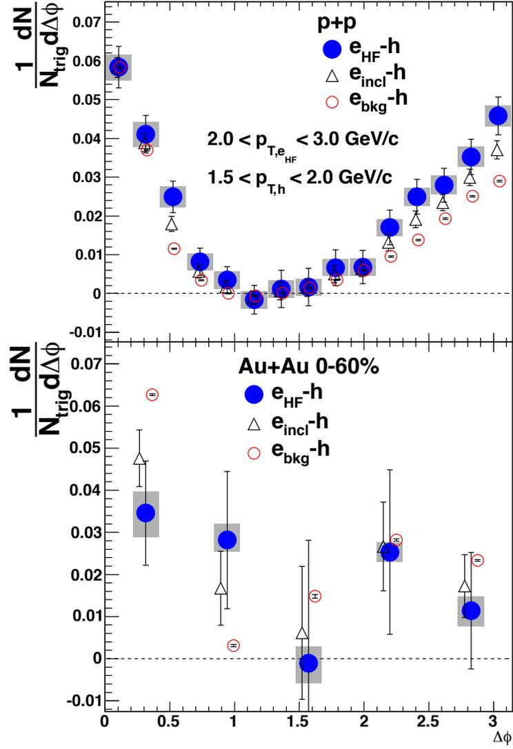
Figure 1.13: Azimuthal correlation of electrons from heavy flavor decays to hadrons in p+p and Au+Au as measured by PHENIX [29].
