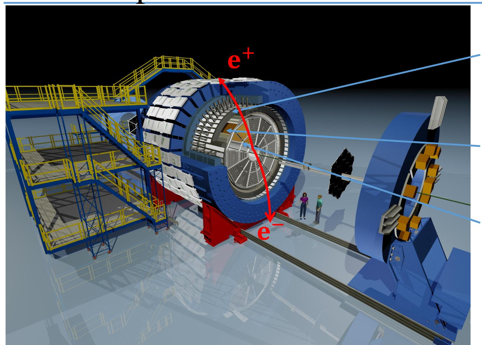
✓ BEMC: Electron identification, trigger
