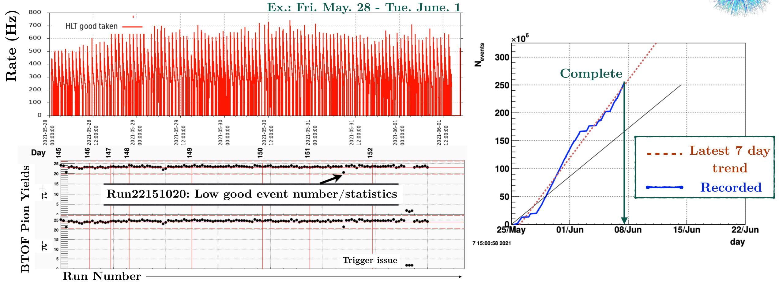
Very consistent fills with minimal downtime and low backgrounds; Average good event rate 450 Hz in latter half of run (improved with machine tuning w.r.t. first few days)
