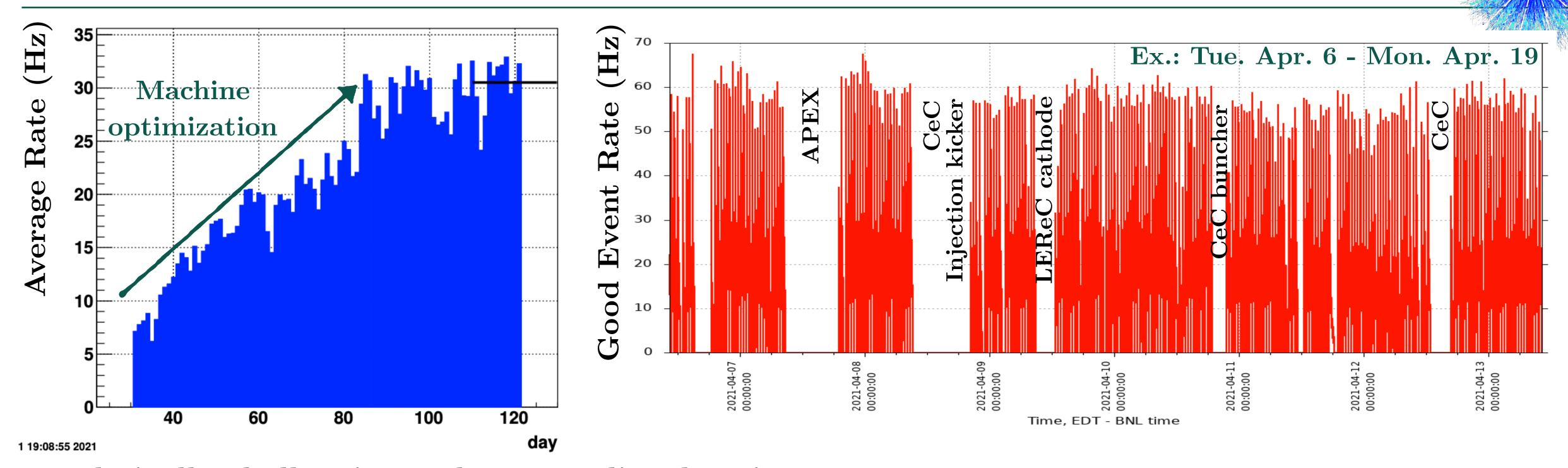
Technically challenging as beam quality deteriorates at low energies; Improved with electron cooling (LEReC)
