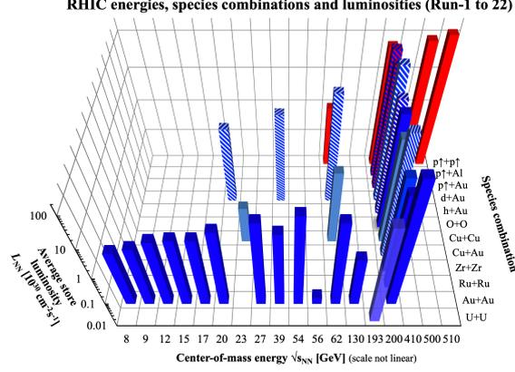
Fig. 1. RHIC average luminosity at various beam species as a function of center of mass energy from Run 1 to Run 22.
