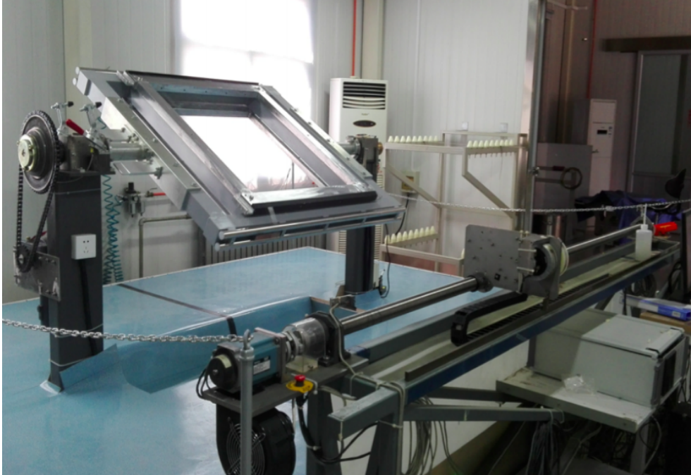
wire pitch and tension controlled by wire winding machine
