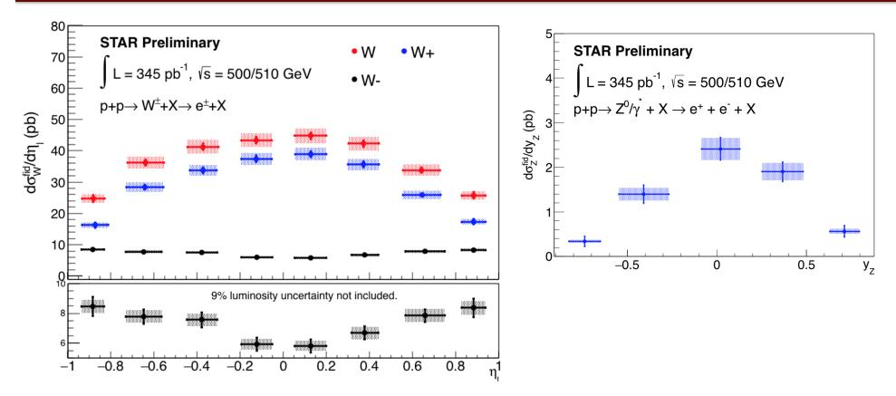
• Including the luminosity (*L*) information, one can also measure the differential cross sections  $\frac{d\sigma^{fid}}{d\eta} = \frac{(N_O - N_B)}{L \cdot \epsilon}$
