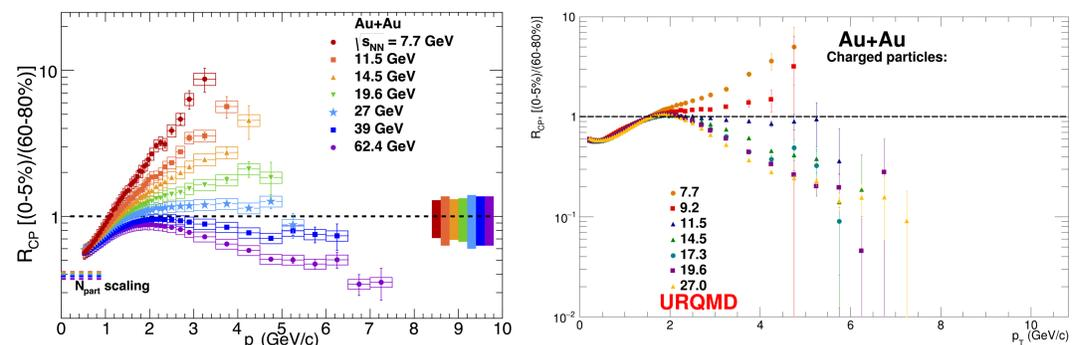
**Figure 1:**  $R_{CP}$  for inclusive charged particles at  $\sqrt{s_{NN}} = 7.7$ -27 GeV collision energies from STAR BES I (left plot) and UrQMD (right plot).
