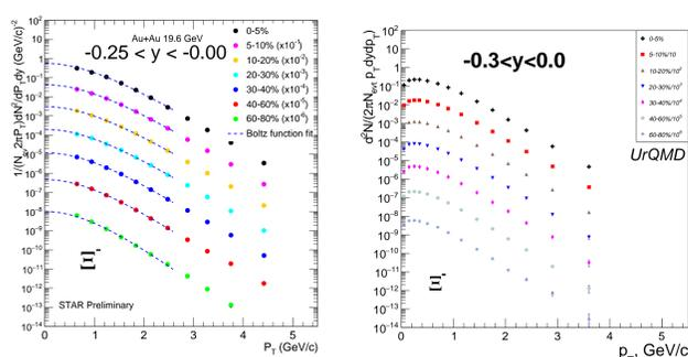
**Figure 2:** Transverse momentum distribution of  $\Xi^-$  for collision energy of 19.6 GeV from STAR BES II (left plot) and UrQMD (right plot). Each spectrum corresponds to a certain centrality class and is multiplied by coefficient from  $1 - 10^6$  for visibility.
