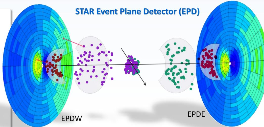
STAR Event Plane Detector is one key upgrade for RHIC Beam Energy Scan-II. A dedicated detector to measure event-plane angle with improved resolution. Two highly segmented EPDs (east & west) cover a pseudorapidity of  $2.1 < |\eta| < 5.1$
