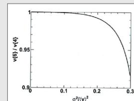
When flow fluctuation is small relatively to the average flow, 6- and 4-particle flows are approximately equal. Higher order harmonics do not provide new information. On the other hand, if flow fluctuation is large in respect to the average flow, 6-particle flow differs from 4-particle flow with Gaussian ansatz.
