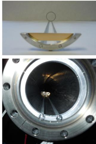
The target foil was held 2 cm below of the beam axis
