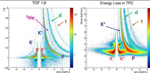
Particle Identification (PID) with STAR Time Projection Chamber (TPC) and Time of Flight (TOF) - outstanding for FXT
