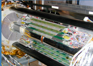
Fig. 2: The SVT, 3 layers of silicon drift detector
