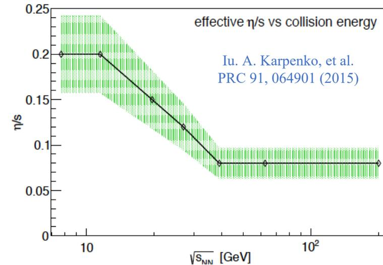
Viscous attenuation ( $\propto \frac{\eta}{s}(T)$ ) is beam energy dependent
