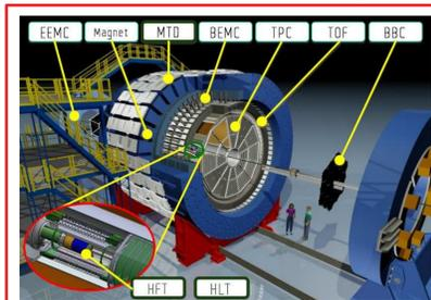
Figure 2: Layout of sub detectors of the STAR experiment.
