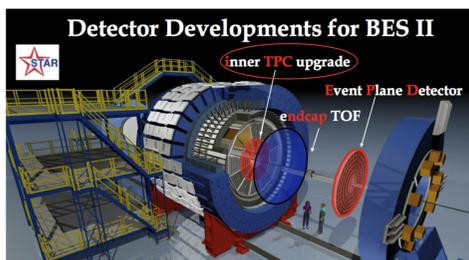
Figure 6: Diagram of the STAR detector<sup>[4]</sup>
