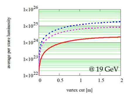
Luminosity upgrade with electron cooling + longer bunch lengths
