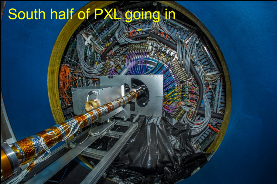
PXL going installed, plumbed, and cabled
