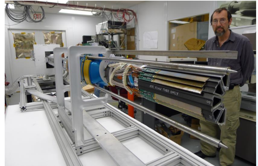
One half pixel with two sectors at test before installation
