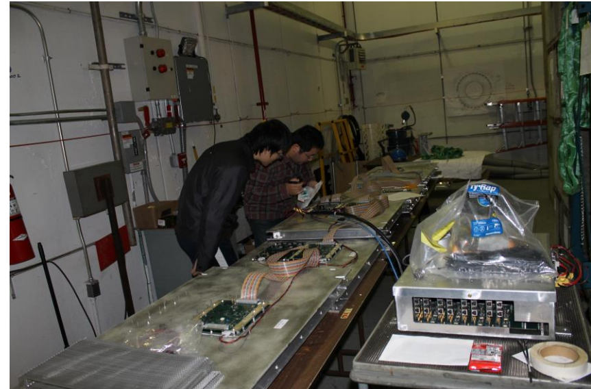
Testing MTD modules prior to installation
