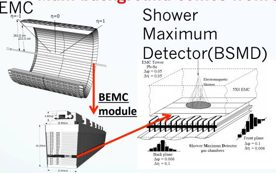
BSMD and BEMC tower used to determine Transverse Shower Profile (TSP)
