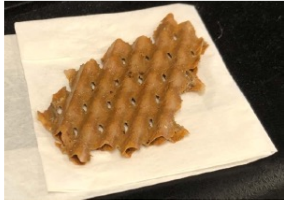
Gunk stuck in the heat exchanger
