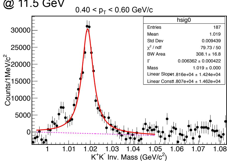
The signal is fitted with a Breit-Wigner function plus a linear residual background after mixed event background subtraction.
