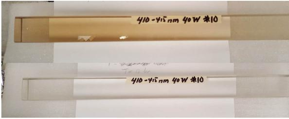
Figure 7–13: Photos of a typically damaged small lead glass cell both before and after curing by means of UV LEDs
