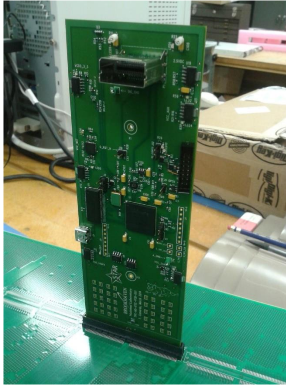
Figure 75: Pre-prototype iFEE (ppFEE) electronic card shown plugged into the padplane
