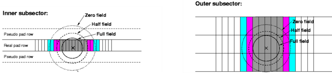
Figure 34: Simulations of the effective pad response function for pads on the inner and outer TPC padplanes. The inner pads were assumed to be 3.35 mm wide and the outer pads 6.7 mm wide. The circles show the 3-sigma limit for the pad response function convoluted with the diffusion limit for particles that drift the full distance from the CM to the padplane. P10 gas is assumed. The different circles show the different response that is recorded when the B field is set to 0.0, 0.25 T, or 0.5 T. [4]
