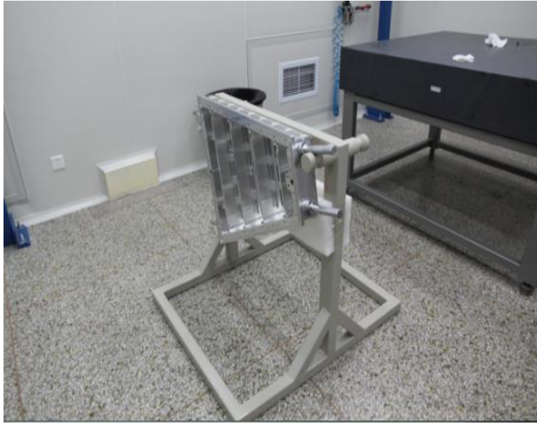
Figure 51: Gluing stand for anode wire mount and granite table.
