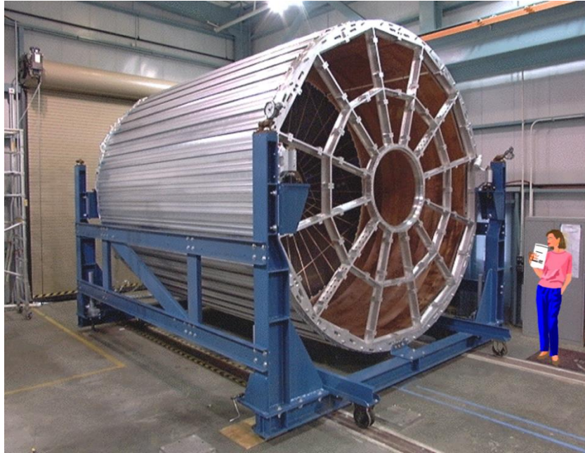
Figure 30: The STAR TPC during construction at LBL. The tracking volume of the TPC is 4 meters in diameter and 4.2 meters long. The photo shows how each end of the TPC is divided into 12 super-sectors and each super-sector is divided into an inner and an outer readout sector.
