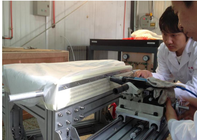
Figure 56: Drilling & pinning on side wire mounts
