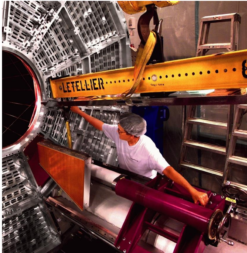
Figure 65: The original sector insertion tool. The sector must fit through the hole in the end-wheel, rotate, and finally pull back into place over a pair of alignment pins (tooling balls) that are located inside the TPC.
