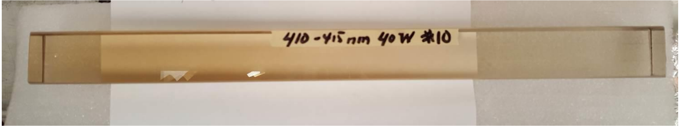
Lead glass cell before cleaning, showing radiation damage
