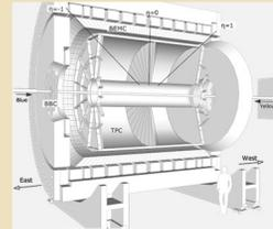
Figure 4. Cross section of the STAR detector showing the TPC and BEMC.
