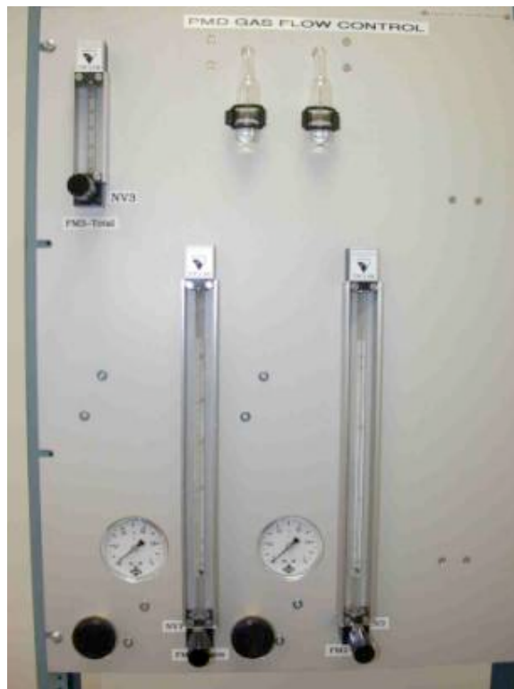
Figure 4.12: Front view of the PMD gas system.
