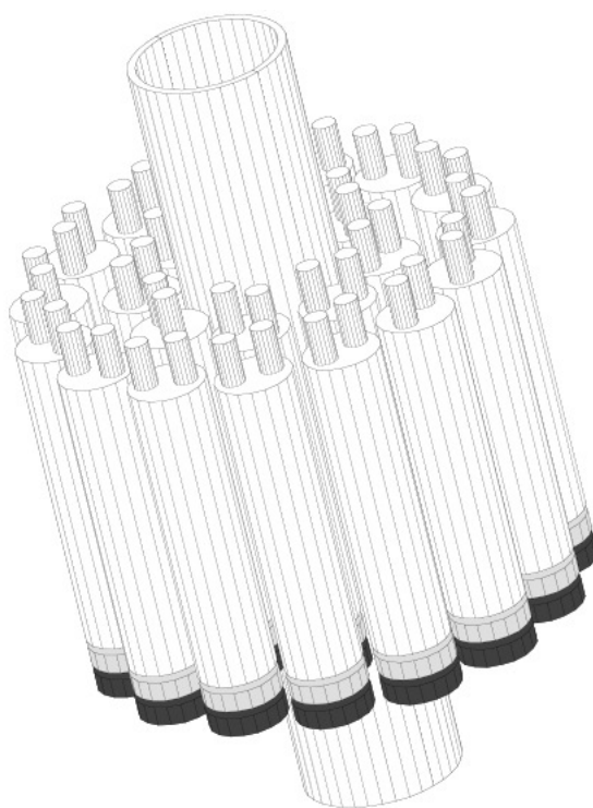
Figure 3.11: Pseudo-vertex position detector (pVPD), with one located on each side of the STAR detector
