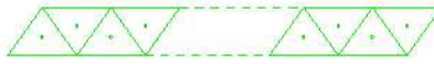
FIG. 7: The SMD planes are built-up from scintillator strips with triangular cross section.
