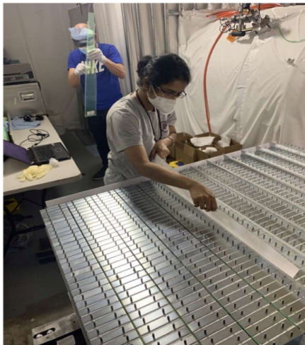
Installing WLS bars
