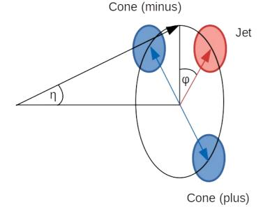
Off-axis cones at  $\pm \, \pi/2$  away in  $\phi$  and at the same  $\eta$
