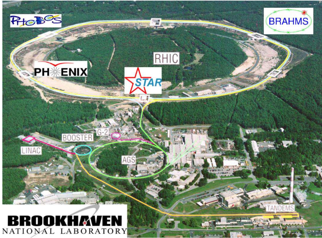
Figure 3.1: The Relativistic Heavy Ion Collider and accelerator chain at Brookhaven National Laboratory (shown in its 2006/2007 configuration).
