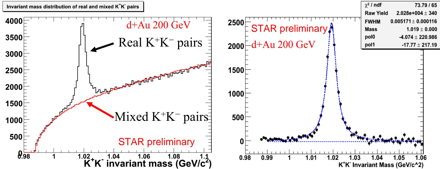
Breit-Wigner + linear function is used to fit  $\phi$  invariant mass distribution after background subtraction
