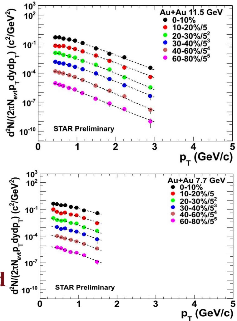
$$\frac{1}{2\pi p_T} \frac{d^2N}{dp_T dy} = dN/dy \frac{(n-1)(n-2)}{2\pi n T(nT + m(n-2))} \left(1 + \frac{\sqrt{p_T^2 + m^2} - m}{nT}\right)^{-n}$$
